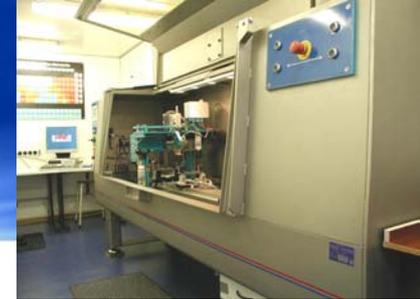
XRF core scanner
